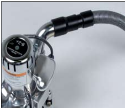
Replace the bag with the hose adaptor and the edger can be easily hooked up to a 1-1/2" vacuum hose.
